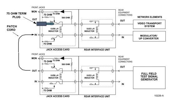
Figure 31. Intrusive Insertion of Test Signal
